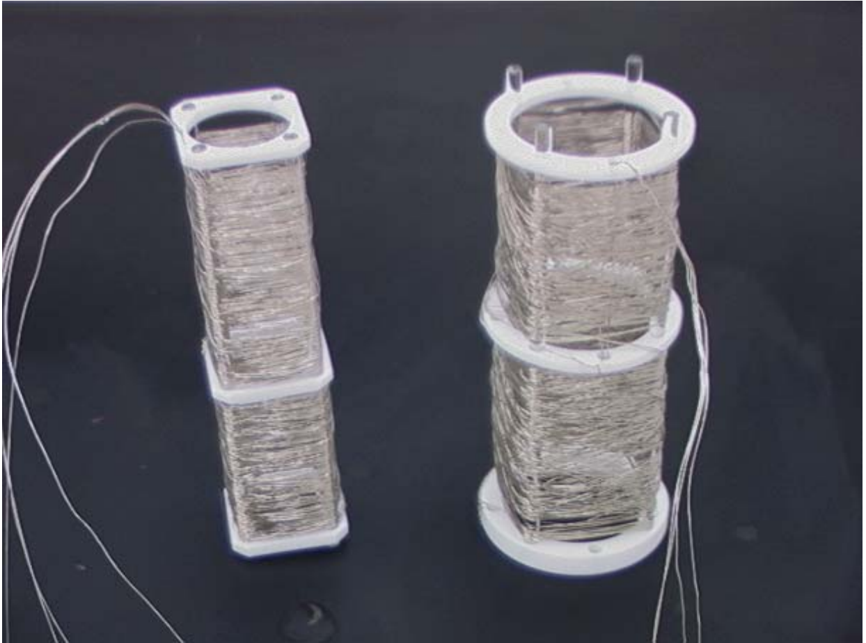
Fig. 2. Nickel wire cathode that fit inside of the nickel wire anode.
